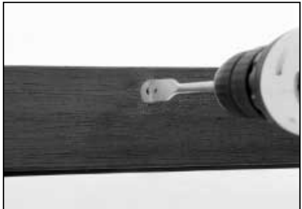
21 Mark drill holes as indicated on both ends of the INSIDE FACE of the sliding door, using a 16mm wood bit. Drill through the first half of the door into the mortise - DO NOT DRILL completely through the door. Place wheels into the mortise with the adjacent slot facing the hole. Screw into position using 1" No 6 screws.
