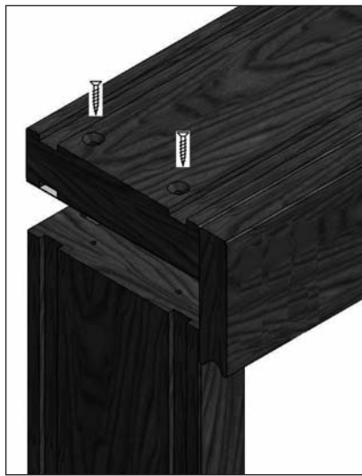
Fig. 2: Head Sub-assembly being fixed to the Jamb Sub-assemblies.
